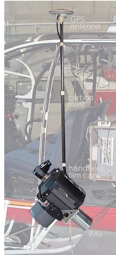
Figure 1. The sensor block.
